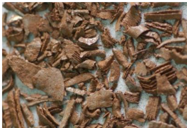
Fig. 1. Fe 0 aggregate catalyst with a flake-like shape obtained from Connelly-GPM Inc., USA.
