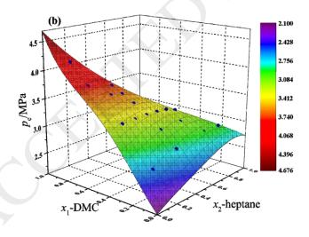
Experimental critical pressures of DMC + n-heptane + n-decane mixture
