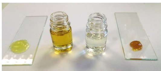
Extraction of lavender flowers by pure CO 2 : 280 bar; 40°C. From left to right: Crude CO 2 extract – Cold filtrated extract – Molecular distillation distillate and residue.
