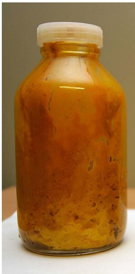
Fig. 1. Total extract of Thymus vulgaris L. linaloliferum . Pure CO 2 @ 280 bar; 45 °C; 12 kg CO 2 /kg feed; Yield (mass basis): 4%.
