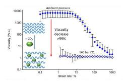
Carbon dioxide and excipient polymers such as poly(ethylene glycol) can be employed to dramatically reduce the viscosity of polymer melt blends and therefore enhance the mixing of thermally labile drugs into formulations for delivery devices.
