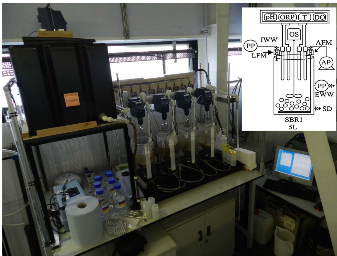
Fig. 1. The configuration of the laboratory-scale SBRs (AFM: air flow meter; AP: air pump; DO: dissolved oxygen probe; IWW: Influent wastewater; EWW: effluent wastewater; LFM: liquid flow meter; ORP: oxidation-reduction potential probe; PP: peristaltic pumps; OS: overhead stirrer; pH: pH probe; SD: sludge draw; T: temperature probe).
