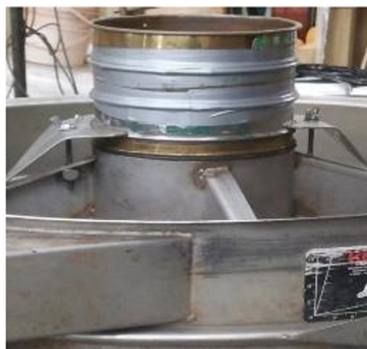
Fig. 1b. The general arrangement used to supply vibration to the fluidized bed.
