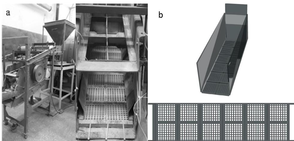
**Fig. 1.** Real (a) and CAD (b) versions of vibrating screen and feeder system.
