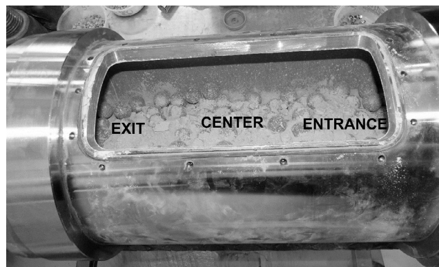
Fig. 1. Interior of the mill during an experiment. Coarse particles are fine compacted aggregates dropped from the window.
