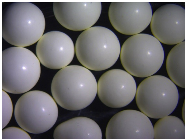
Fig. 1. MINERAX ceramic beads (75% Alumina 25% Zircon).
