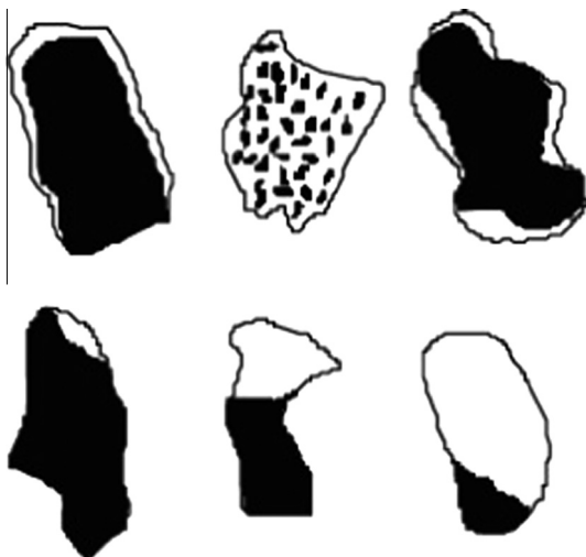
Fig. 1. Example of binary particles with complex texture (top row) and simple texture (bottom row) (Lastra, 2002).
