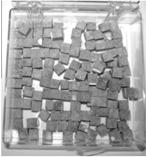
Fig. 1. Cubic copper sulfide ore specimens (6 × 6 × 6 mm) from the United States.
