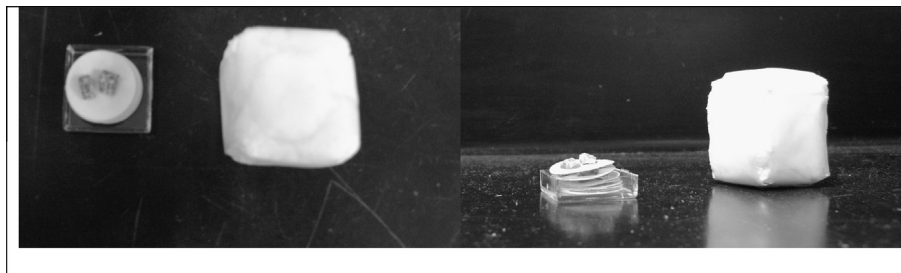
Fig. 2. Progeny particle size classes mounted on labeled filter papers and stacked in a cylindrical styrofoam container for CT scans.
