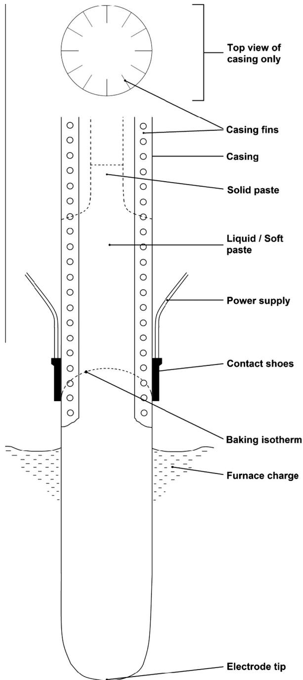
**Fig. 1.** Simplified representation of a Söderberg electrode, adapted from Arnesen et al. (1979). The main figure at the bottom indicates a side sectional view of the electrode, while the top image indicates the top sectional view of the casing only.
