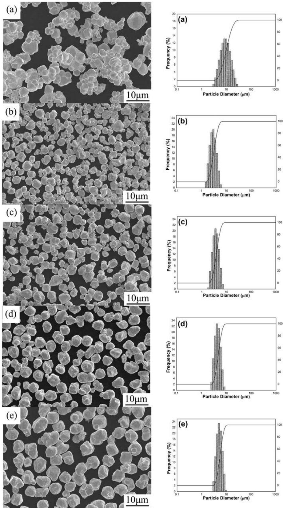
**Fig. 1.** SEM photographs of surface morphology and particle size distribution of W powders at different rotating speed: (a) as-received powder; (b) 4200 rpm; (c) 3500 rpm; (d) 3150 rpm; (e) 2800 rpm.
