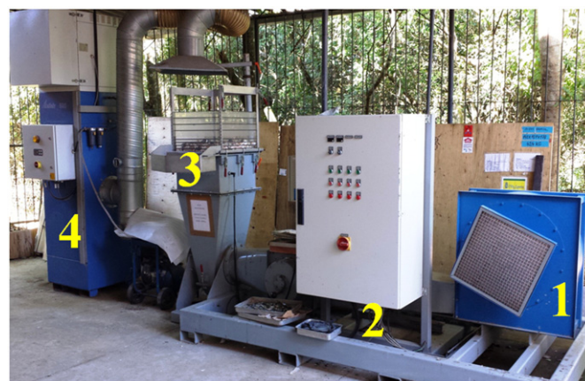
Fig. 1. Air jig model AllAir® S-500 from AllMineral. (1) Feeding unit; (2) control panel; (3) separation chamber; (4) powder filtering unit.
