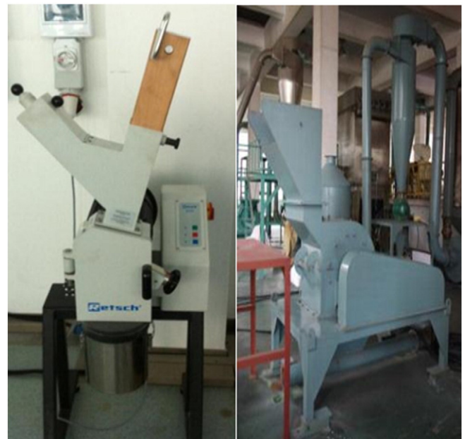
Fig. 3. Instrument for size reduction. (left: Retsch SM2000; right: Fengli CSF570).
