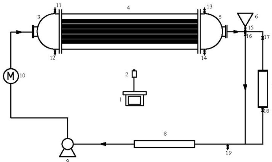
Fig. 1. Schematic diagram of the horizontal multi-tube circulating fluidized bed system. 1—computer; 2—CCD; 3—front shell cover; 4—horizontal tube bundle; 5—rear shell cover; 6—loading hopper; 7—particle collection section; 8—the horizontal single tube; 9—centrifugal pump; 10—electromagnetic flowmeter; 11–19—ball valves.
