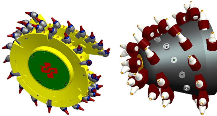
Fig. 1. Shearer drum and cutting head of road-header.
