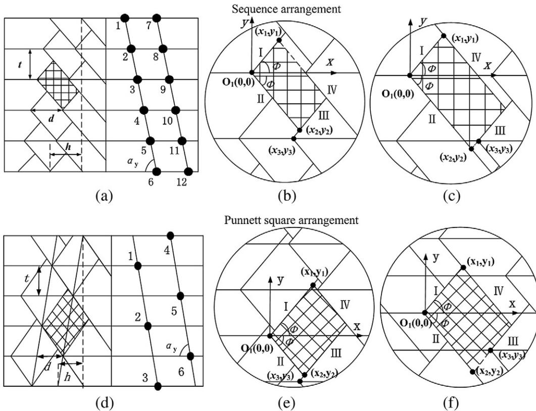
Fig. 2. Breakout patterns of two different pick arrangements.
