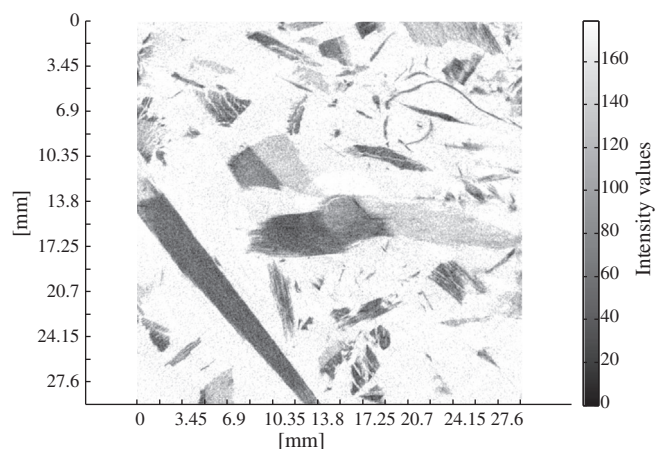
Fig. 2. Sample of a scanned section of sawdust packing ( W_1 , 850 \times 850 pixels).
