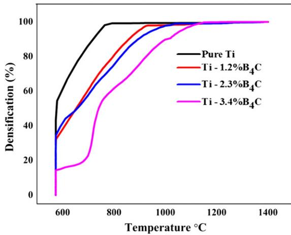
Fig. 2. Densification curves of titanium and Ti/B<sub>4</sub>C powder mixture sintered at 30 min.
