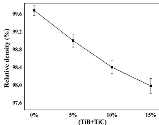
Fig. 1. Relative density of titanium and Ti/(TiB + TiC) composites sintered at 30 min.
