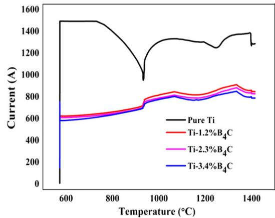
Fig. 3. Current curves of titanium and Ti/B<sub>4</sub>C powder mixture sintered at 30 min.
