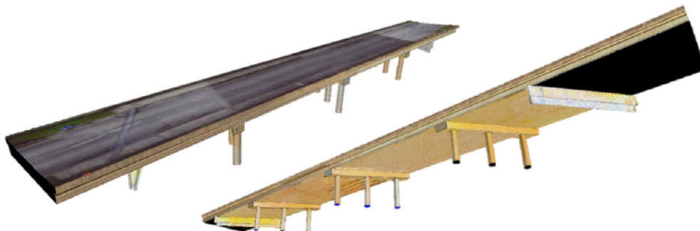
Fig. 1. 3D as-is model of fully-textured RC highway bridge, deck view on the left, bottom view on the right.
