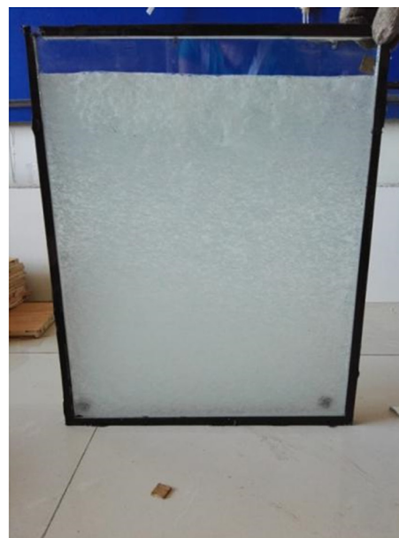
Fig. 1. PCM-filled glazed roof unit (left: liquid state; right: solid state).
