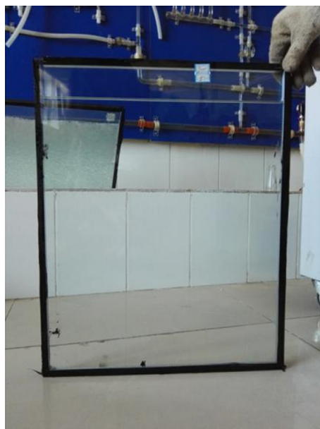
Fig. 1. PCM-filled glazed roof unit (left: liquid state; right: solid state).
