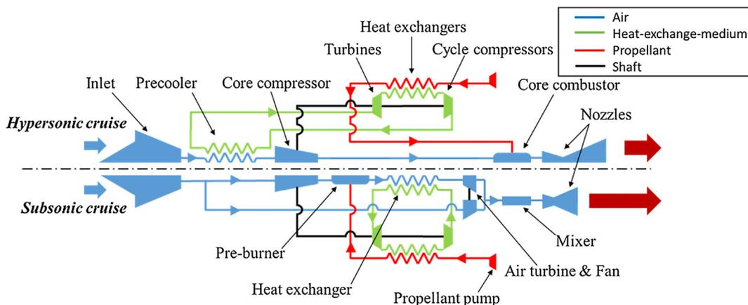
Fig. 1. The operation mechanism and basic structure of HPCCE [13].
