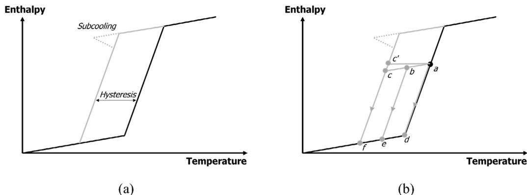
Fig. 1. (a) Hysteresis and subcooling in a PCM melting and solidification process. (b) Scenarios for modelling the transition between heating and cooling in a partially melted PCM. Based on [19].
