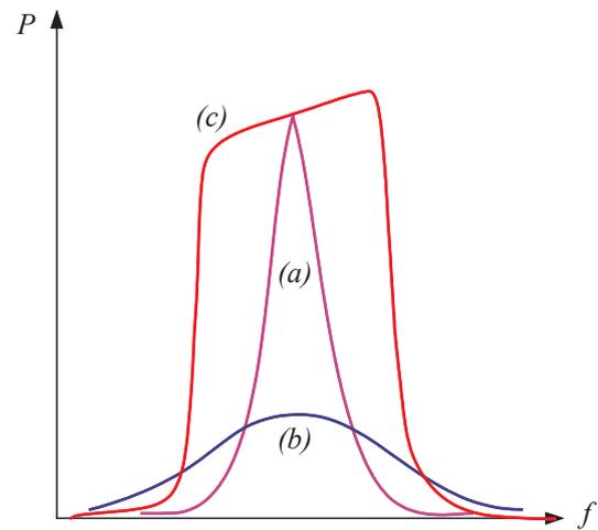
Fig. 1. (a) High NPD with high-Q; (b) broad bandwidth with low-Q; and (c) all-round performance with both decent power output and broad bandwidth can be achieved from a gap-closing scheme with high-Q from low packaging pressure (without increasing the acceleration amplitude).
