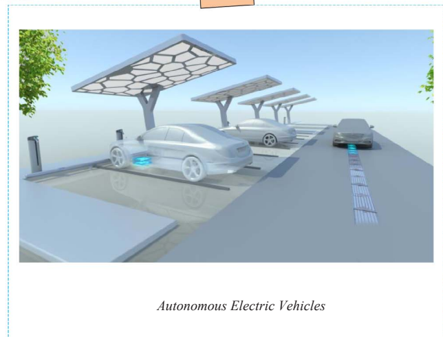
Fig. 1. Future energy highway integrating inductive coils for both inductive power transfer and induction heating, with green energy technologies for (autonomous) electric mobility.
