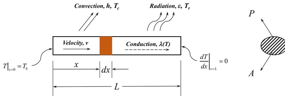
Fig. 1. Schematic diagram of convection and radiation from the surface of a moving rod.
