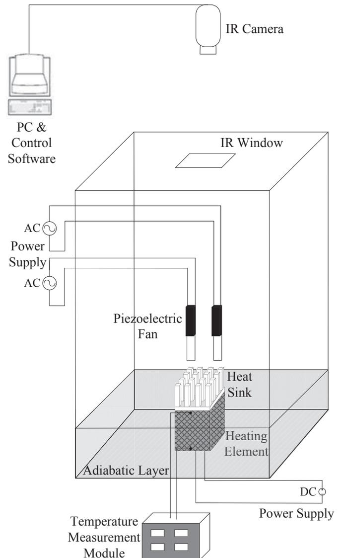
Fig. 1. Schematic diagram of experimental apparatus.
