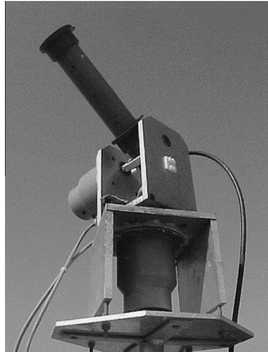
Fig. 1. Sensor of sensor based dual-axis solar tracker equipped with a radiance limiting tube, and mounted on an independent dual-axis mechanical system [39].
