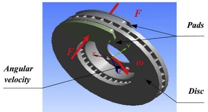
Fig. 1. Disc-pads assembly with forces applied to the disc.
