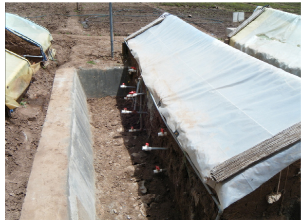
Fig. 1. Nine sampling ports in the side of one of the test digesters at K'ayra.
