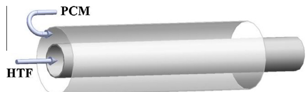
Fig. 1. Schematic of the shell-and-tube phase change thermal energy storage unit.
