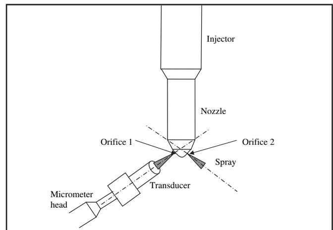
Fig. 1. Schematic of the spray impingement technique.
