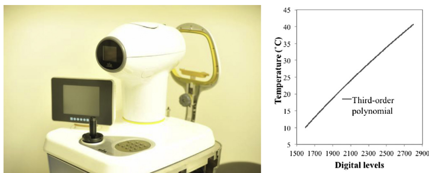
Fig. 1. Customized ocular surface thermography. A. Photograph of the customized ocular surface thermography. B. Third-order polynomial transfer function used to convert digital value into temperature value.
