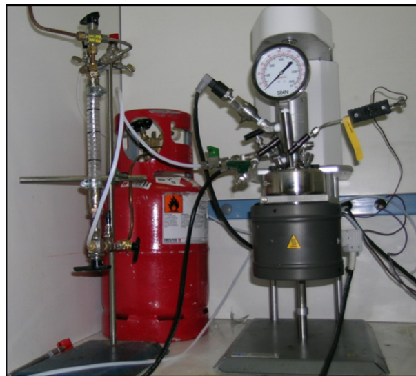
Fig. 1. Experimental set-up for catalytic etherification of glycerol.
