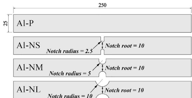
**Fig. 1 – Geometry of plane and notched specimens (dimensions are in mm).**
