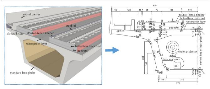
Fig. 1 - Typical section and temperature gauges of Chinese HSR bridge-track system (cm).
