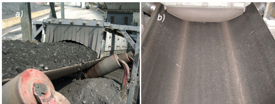
Fig. 2 – Typical problems due to the incorrect belt bending stiffness of conventional trough conveyors: (a) Excessively stiff belt causes spillage of the material; (b) excessively flexible belt causes damage of the belt, observed as two wear lines, due to the idler junction failure.
