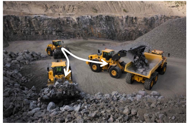
Fig. 1. A wheel loader performs a “short loading cycle” in blasted rock from face, as a part of a production chain [31].
