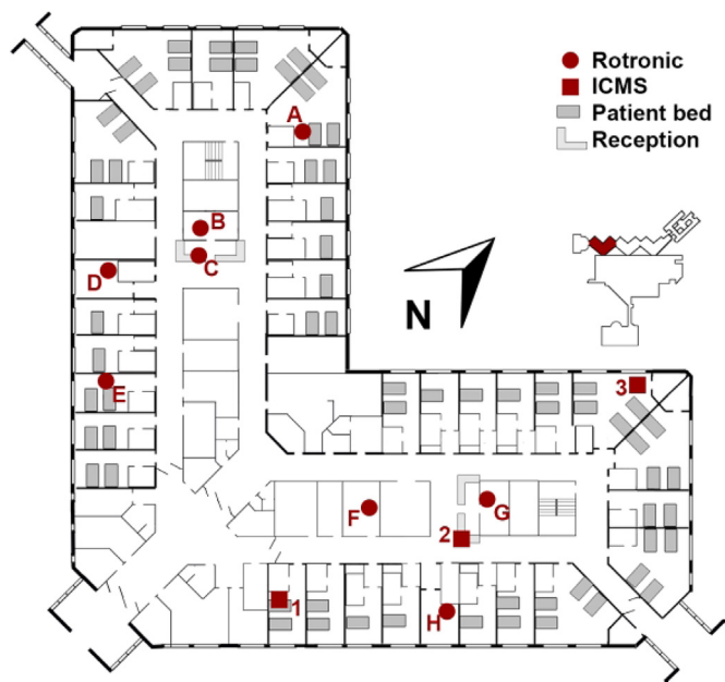
Fig. 1. Floor plan of the wards, east and west, where the study was undertaken. A–H: locations of the 8 Rotronic sensors. 1–3: locations of the 3 indoor climate measurement stands (ICMS).
