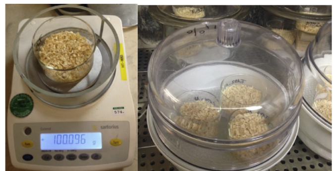
Fig. 1. Samples in glass dishes (left) and desiccators (right) for sorption measurement within hygroscopic range.
