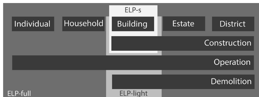
Fig. 1. The different activities and levels included in the ELP [6,7,21]. The dark background represents the full ELP, the lighter background the simplified version for building level, ELP-light. The white background represents the simplified ELP of building structures (ELP-s), which is tested in this study.
