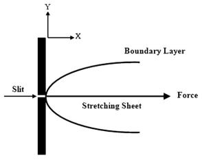
Fig. 1. Physical model and coordinate system.
