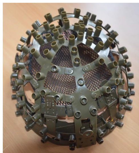
Fig. 3. Inner structure of the helmet.
