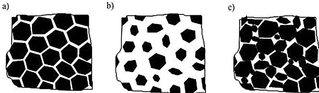
Fig. 1. Different types of two-phase MCC internal structures: (a) with small thickness and continuous interfaces, (b) with dilute distribution of ceramic grains in metallic matrix, (c) with not continuous interfaces.
