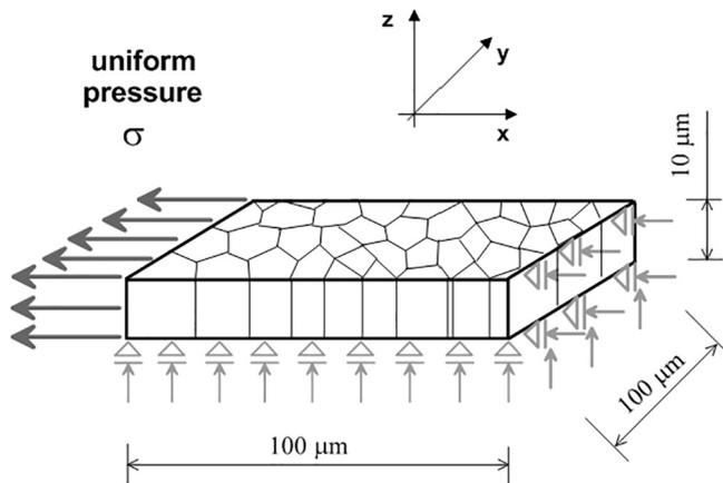
Fig. 3. Loading and boundary conditions of the RVE.
