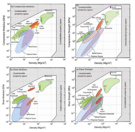
Fig. 1. Modified Ashby material strength versus density map for engineering materials [8].
