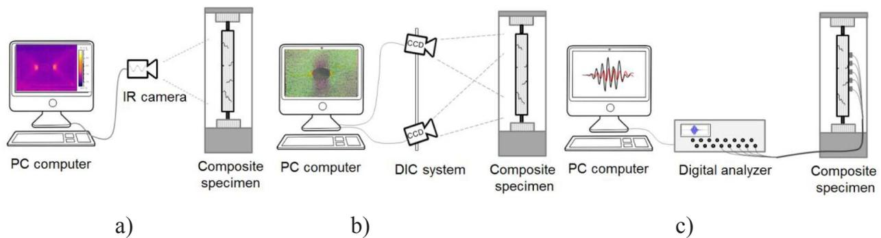
Fig. 1. Schematic set-up of experimental NDT techniques: a) thermal (passive thermography), b) visual (DIC), c) ultrasonic (SHM).
