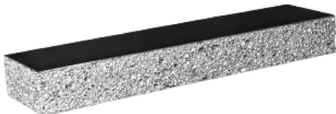
Fig. 2. Three-layer beam with a metal foam core.
