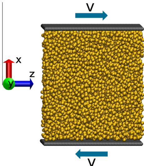
**Fig. 1.** Simulation setup of the MRF shear cell. The walls are modeled as an ensemble of overlapping spherical particles. They are moved in  $z$ -direction with velocities  $\pm \mathbf{v}$ . Confined between the walls are the randomly distributed magnetic particles. The carrier fluid is not displayed.
