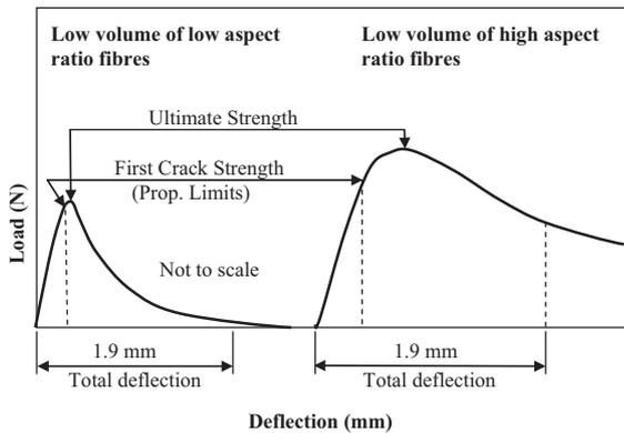
Fig. 3. Effect of fibre volume on the load vs. deflection behaviour of FRC [2].
