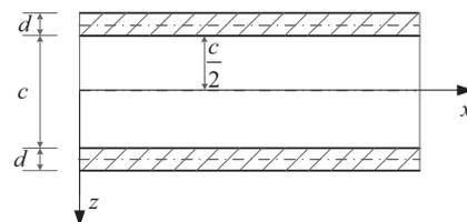
Fig. 1. A symmetric sandwich panel.
